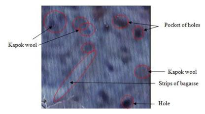
Figure 14 Micrograph of bagasse-Kapok interwoven structure showing pocket of holes (×150)
