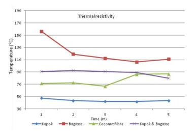
Figure 12 Thermal resistivity of base materials
