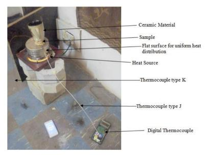
Figure 9 Experimental setup
