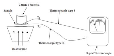
Figure 8 Schematic diagram of thermal diffusivity
