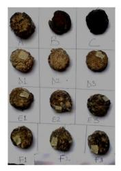
Figure 5 Moulded biomass composites
