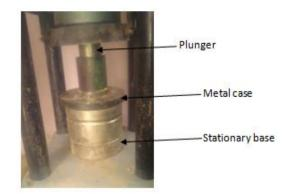
Figure 4 Biomass composite under Compression
