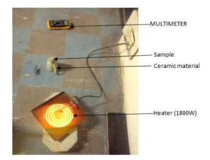
Figure 7 Setup of thermal conductivity test
